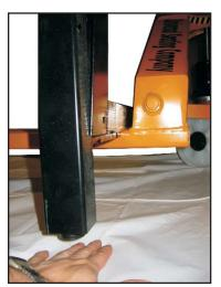
When the hydraulic cart is raised, the entire booth frame is off the floor with plenty of clearance.
